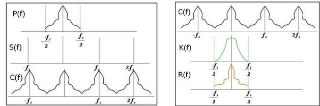
**Fig. 1.** In the frequency domain, sampling (left) and reconstruction (right) of a single scan-line for a single projector. Left: The signal  $P(f)$  bandlimited by  $\frac{f_s}{2}$  is convolved with the sampling signal  $S(f)$  to generate the sampled signal  $C(f)$ . Right: The sampled signal  $C(f)$  is multiplied by the reconstruction kernel  $K(f)$  of width  $\frac{f_s}{2}$  to reconstruct the bandlimited signal  $R(f)$ .
