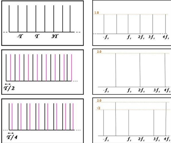
**Fig. 2.** Left: In the spatial domain, the sampling function  $S(f)$  from a single projector separated by pixel width  $T$  (top), the sampling function  $S_o(f)$  for interleaving of pixels for a scan-line from two overlapping projectors (one in black and another in pink) shifted by  $\frac{T}{2}$  (middle),  $\frac{T}{4}$  (bottom). Right: The corresponding frequency response of the sampling functions on the left.
