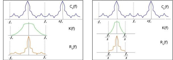
**Fig. 4.** In frequency domain, reconstruction using a kernel of support  $f_s$  (left) and  $\frac{f_s}{2}$  (right) of the super-resolution signal  $P_o(f)$  sampled by two overlapping projectors interleaved by a distance  $\frac{T}{2}$ . For each, the sampled signal  $C_o(f)$  (top) is multiplied by the reconstruction kernel  $K(f)$  (middle) to generate the reconstructed signal  $R_o(f)$  (bottom).
