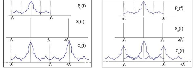
**Fig. 3.** In frequency domain, sampling of a super-resolution scan-line  $P_o(f)$  by  $S_o(f)$  from two overlapping projectors with their pixels interleaved by  $\frac{T}{2}$  (left) and  $\frac{T}{4}$  (right). In other word, the super resolution signal  $P_o(f)$  (top) is convolved sampling signal  $S_o(f)$  (middle) to generate sampled signal  $C_o(f)$  (bottom).
