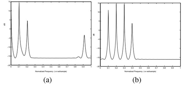
**Fig. 5.** (a) The standard Volterra filter output *psd* estimation and (b) PWM filter output *psd* estimation
