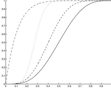
**Fig. 3.** The *bdp* of a single WM with  $x_i$  inputs, second-order PWM filter with  $x_i$  and  $x_i^2$ , second-order PWM filter with  $x_i$ ,  $x_i^2$ , and  $x_i x_j$ , and standard second-order Volterra filter, are represented in solid line, dashed line, dotted line and dash-dotted line respectively, for  $N=7$
