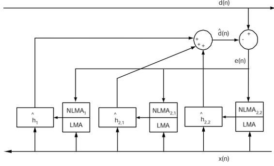
**Fig. 2.** The PWM filter coefficients optimization with the Normalized fast LMA
