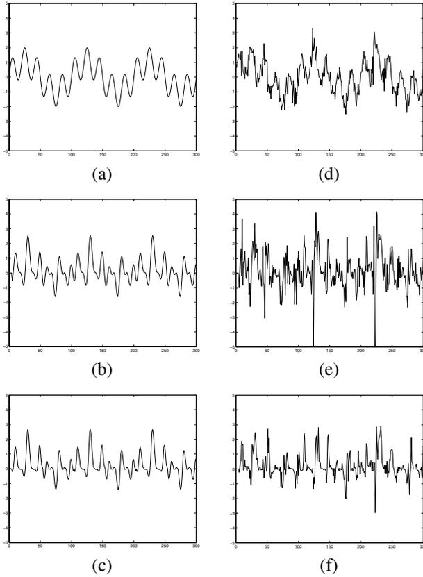
**Fig. 4.** (a) is noise-free input signal, (b) standard Volterra and (c) PWM filter output, (d) noisy input signal ( $\mathcal{L}$  with  $\sigma^2=0.25$ ), (e) standard Volterra and (f) PWM filter output for noisy input
