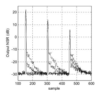
**Fig 1.** Output NSR  $(\sigma_e^2 / \sigma_d^2)$  for 3 normalised LMS algorithms:  $\nabla = \text{NMLS}$ ; o = equation (5);  $\Delta = \text{equation}$  (6). Learning curves averaged over 100 trials. M = 9. Input spike amplitudes +8, 0 and -8 dB w.r.t.  $\sqrt{M}\sigma_x$ , at samples number 150, 300 and 450.
