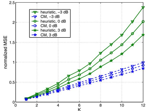
**Fig. 2.** MSE vs.  $K$  for different SNR (angular spread  $10^\circ$ ,  $f_d = 0.12$ ).
