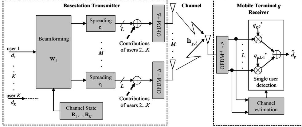
Figure 1: Proposed MC-CDMA downlink system with transmit beamforming.
