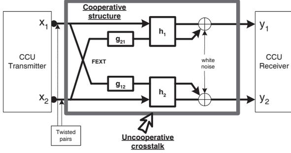
Fig. 1 . MIMO-CCU for  $N = 2$
