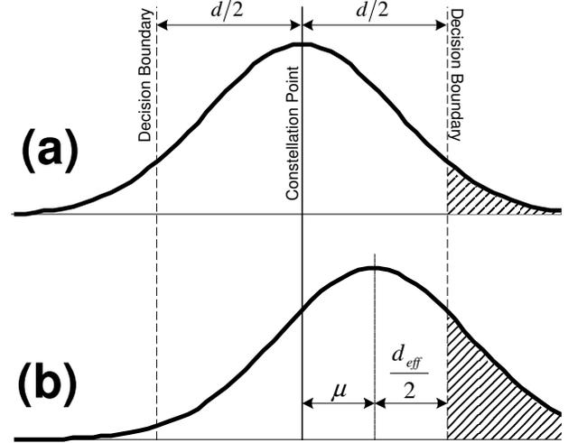
Fig. 1- Probability density functions of (a) an unbiased Gaussian, and (b) biased Gaussian noise sources. The highlighted area indicates the probability of receiving a data point out of the decision boundary, hence the probability of error.
