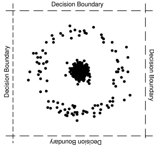
Fig. 2- The error scatter plot when the communication channel suffers from both Gaussian and impulse noise sources. The cluster of points at the center represents the effect of Gaussian noise when impulse noise is not active. The outer ring shows the impact of impulse noise.
