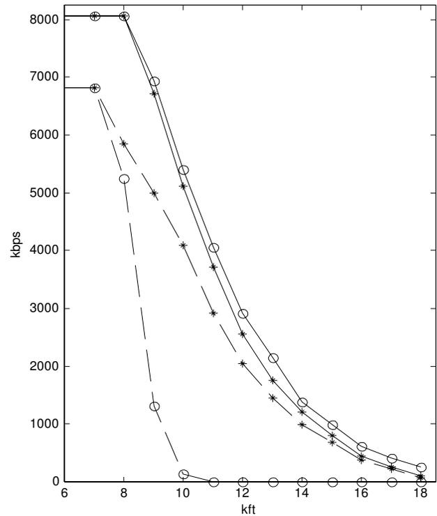
Fig. 4- Data rate versus loop length in presence of impulse noise. Solid and dashed lines indicate the bit rate at physical layer and the average FTP throughput, respectively. Stars and circles mark the rates with and without impulse compensation, respectively.
