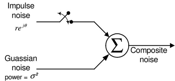
Fig. 3- A noise model that combines the effects of background Gaussian noise and the impulse noise.
