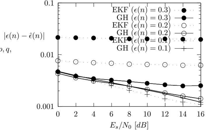
Fig. 1. Absolute frequency offset estimation error.
