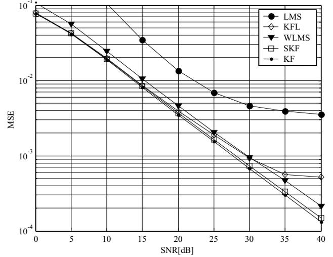
**Fig. 1.** Steady-state MSE versus SNR. Simulation for LMS, KFL, WLMS, SKF and KF tracking over Clarke model channel ( $W = 8$ ,  $P = 5$ ,  $\tau = [1 \ 2.1 \ 2.4 \ 4.1 \ 4.5]T$ ,  $\sigma_i^2 = \sigma^2 2^{-i}$ ).
