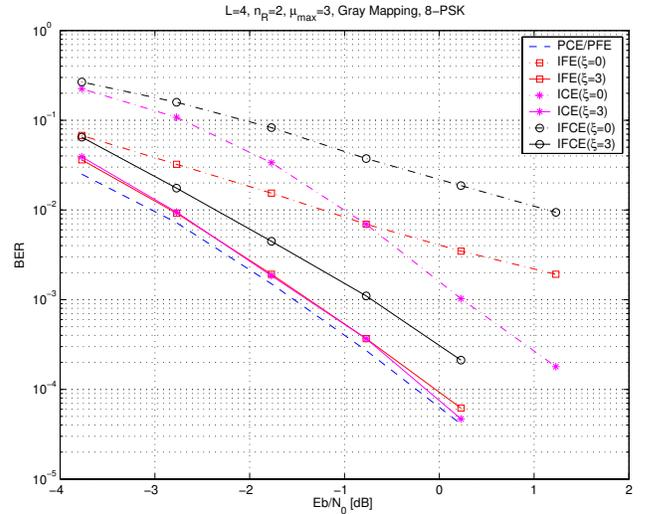
**Fig. 2.** BER-performance for different estimation scenarios. (PCE/PFE: perfect synchronization, IFE: estimation of frequency offset only (channel known), ICE: estimation of channel only (frequency known), IFCE: both frequency and channel estimation)
