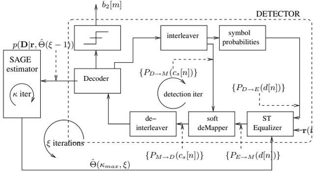
**Fig. 1.** Receiver structure.
