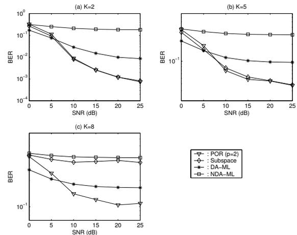
Fig. 4. BER comparison based on channel model CM2.
