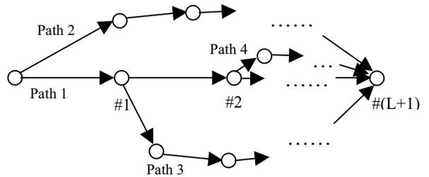
Figure 3: Partially Disjoint Multi-Path of Serial Relays (PDMP-SR)
