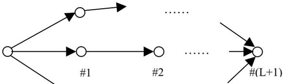
Figure 2: Completely Disjoint Multi-Path of Serial Relays (CDMP-SR)
