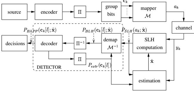
Fig. 1. BICM-ID system with embedded estimation.
