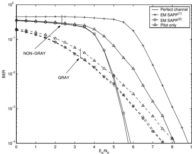
**Fig. 3.** Bit error rate performance of the iterative detector with embedded estimation of  $A$  and  $\theta$ .
