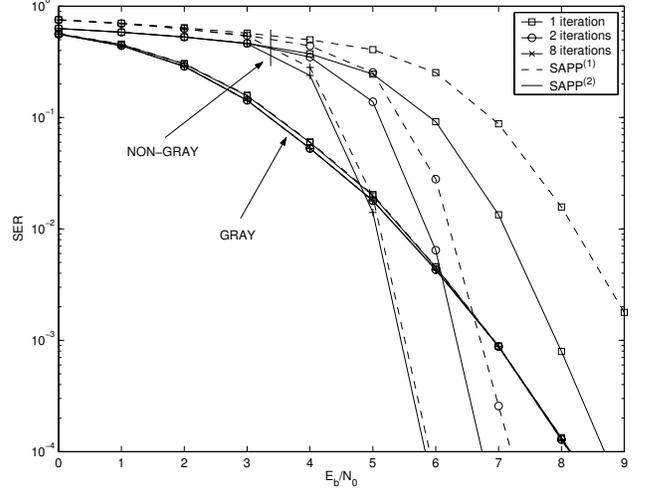
Fig. 2. Symbol error rate based on the a posteriori symbol probabilities for a perfectly synchronized system.
