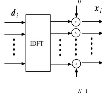
Fig. 2. Alternative implementation of circular precoder
