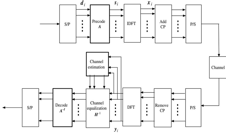
Fig. 1. OFDM system with linear precoder
