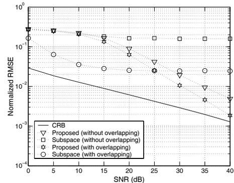
**Fig. 3.** Normalized RMSE of the CRB, proposed and subspace blind channel estimates versus SNR, for  $K = 48$ ,  $L = 3$ ,  $N = 2$  and  $SIR = 10\text{ dB}$ .
