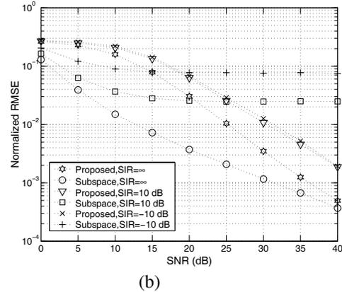
**Fig. 2.** Normalized RMSE of the proposed and subspace blind channel estimates versus SNR and SIR, for  $K = 48$ ,  $L = 3$  and  $N = 2$ . (a) No overlapping. (b) Overlapping.
