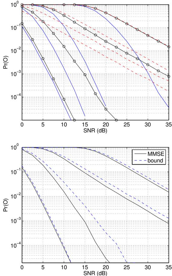
**Fig. 2.** Joint spatial encoding. Top: Unconstrained receiver (solid line), MMSE-LE (solid line with  $\circ$ ) and ZF-LE (dashed line). Bottom: MMSE-LE and the upper bound (17). From left to right  $R=1,2,4,10$  bits/sec/Hz.
