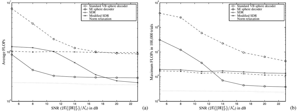
Fig. 2. Average and worst-case complexity performance of the SDR and sphere decoding algorithms.
