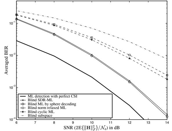
**Fig. 1.** BER performance in a 4 receiver antenna case.
