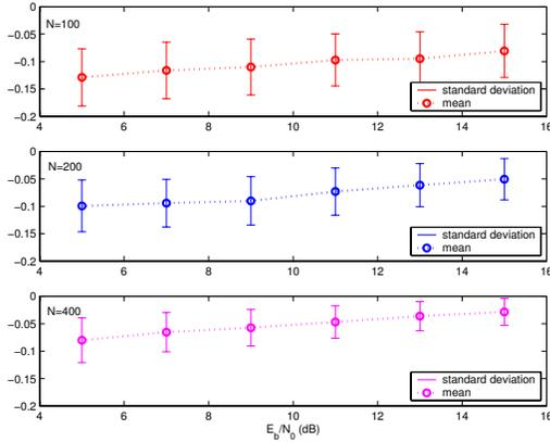
**Fig. 3.** Normalized (with respect to  $T_s$ ) mean  $\pm$  half of the standard deviation of the timing estimation errors when both MUI and ISI are present (MUI is caused by two asynchronous nodes with the same power).
