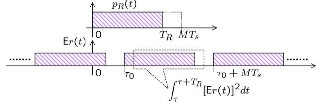
**Fig. 2.** Schematic illustrating the energy detector used for timing estimation.
