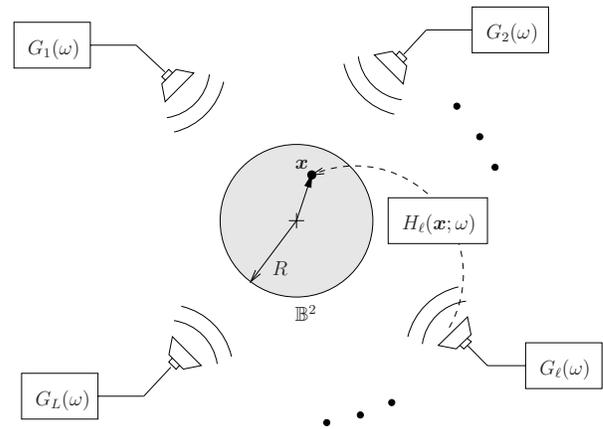
**Fig. 1.** Use of  $L$  loudspeakers to reproduce a desired field in a control region  $\mathbb{B}^2$  with loudspeaker signals  $G_\ell(\omega)$  and ATFs  $H_\ell(x, \omega)$  from the  $\ell$ th loudspeaker to point  $x \in \mathbb{B}^2$ .
