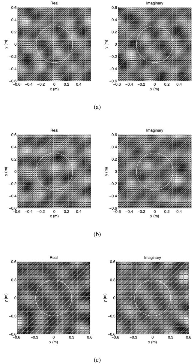
**Fig. 2.** Reproduction of a plane wave for (a) a free field, (b) the same free field design in the reverberant room, and (c) a reverberant design in the reverberant room. Percentage reproduction errors are 0.87%, 307% and 0.85% respectively.
