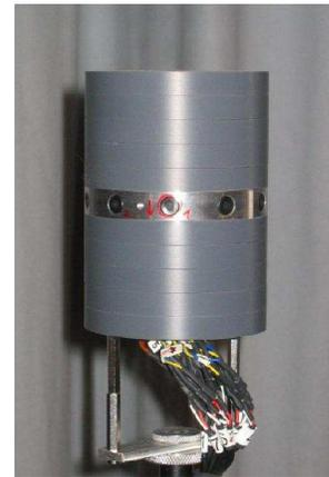
**Fig. 5.** Photograph of the ten-element microphone array system with  $R = 0.04$  m
