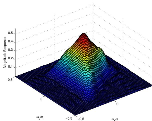
**Fig. 2.** Magnitude frequency response of  $15 \times 15$  two-dimensional filter.
