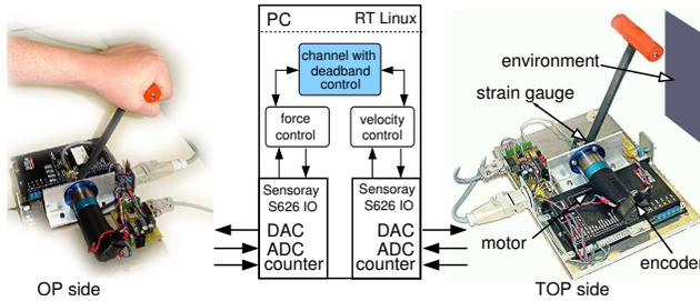
Fig. 3. Experimental setup with two 1-DOF haptic devices
