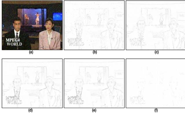
Figure 2. Estimated luminance errors of relevant filters for 1<sup>st</sup> frame News corrupted by 4% impulse noise: (a) noisy image, (b) VMF, (c) AMSF, (d) BVDF, (e) GVDF, and (f) HIMDF (available in large images at [11]).
