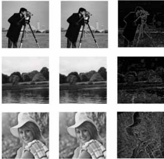
(a) carrier images (b) stego-images (c) difference images (amplified 30 times)
