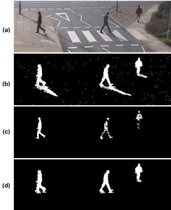
**Figure 3.** Illustration of the shape reconstruction process for the foreground regions. (a) the incoming image; (b) the “mask” image from initial segmentation; (c) the “marker” image after shadows/highlights removal, and (d) the final reconstructed objects shapes.
