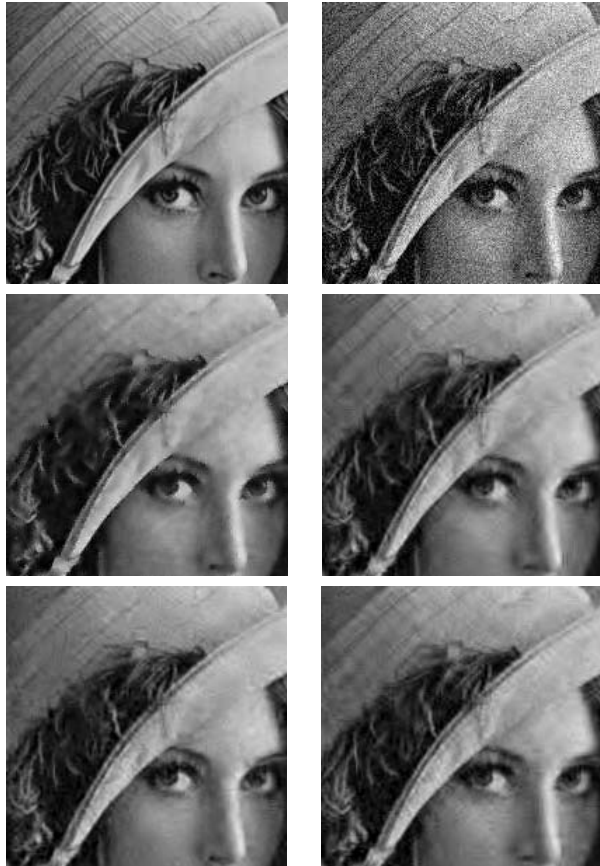
Fig. 2. Details from image Lena. Top line from the left; original and noise added ( \sigma^2 = 400 ). Second line; Wiener with 5 \times 5 mask and DWT coiflet5. Last line; frame with G=db4 and frame with G=coiflet5.
