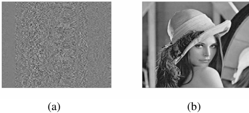
Fig. 3: The output of the observation filter and the reconstructed image. The PSNR of the reconstructed image equals 37.05
