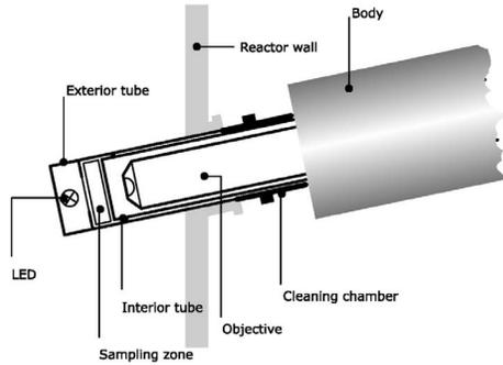
**Fig. 1.** In-situ microscope.
