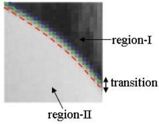
**Fig. 2.** 1D manifold constraint of line singularities: red, green and blue colors denote positive, zero and negative distances from the contour respectively.
