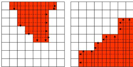
**Fig. 4.** Modified SA-DCT without row/column shifting (transform goes along solid lines first and then dashed).
