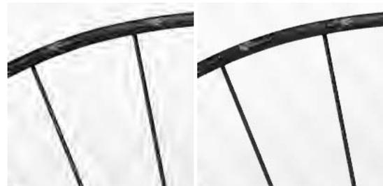
**Fig. 8.** Comparison of portions of decoded *bike* images by SPIHT (left,PSNR=25.05dB) and our baseline coder (right, PSNR=28.69dB) at the same bit rate of 0.192bpp.
