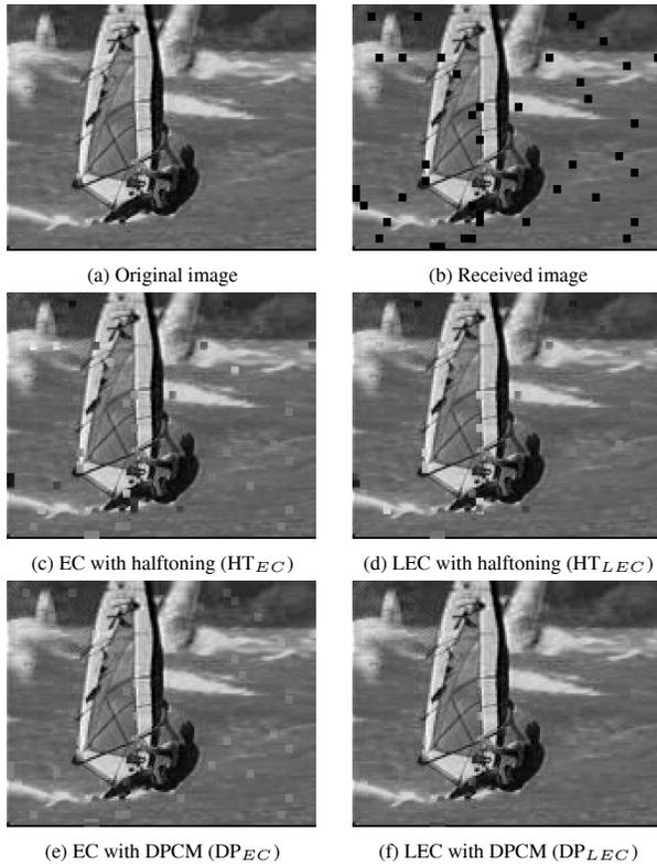
**Fig. 3.** The received image is obtained for a mean packet loss probability of 0.15 and variance 2.5%. The PSNR values of the images are (b) 20.2943, (c) 27.3112, (d) 30.8620, (e) 28.8613, and (f) 33.1337. The value of  $\alpha$  used in both cases was 3.
