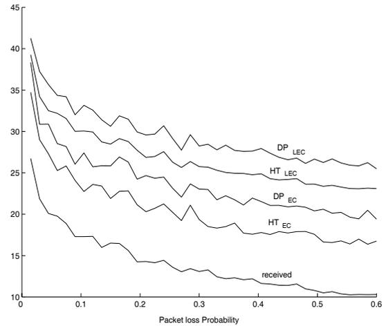
**Fig. 4.** PSNR vs. loss rate curves of ECDH with halftoning and ECDH with DPCM encoding.
