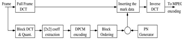
Fig. 1. Block diagram of the embedding algorithm.
