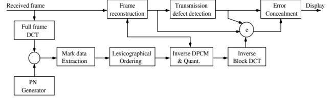
Fig. 2. Block diagram of the retrieval algorithm.
