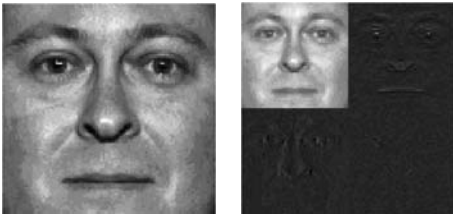
Fig. 2: Left: original image; Right: the 1-level wavelet decomposition.
