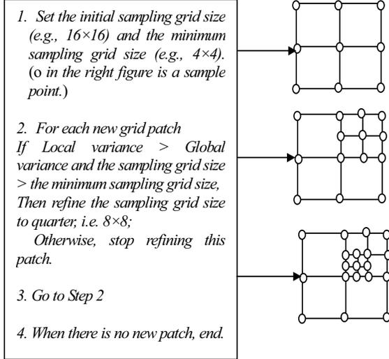
Figure 3. Non-uniform sampling algorithm
