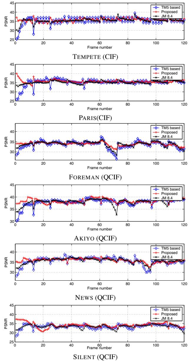
**Fig. 2.** psnr vs. frame for three rate control algorithms.
