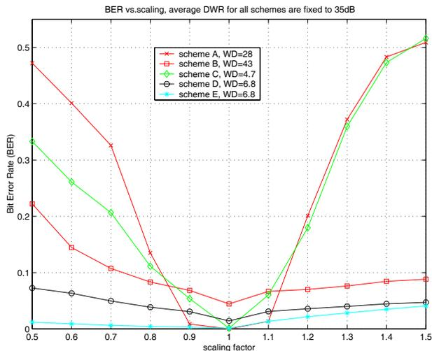
Fig. 4. Robustness versus amplitude scaling
