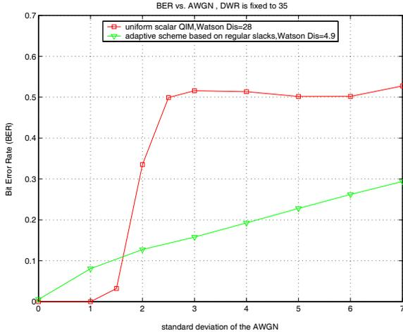
**Fig. 3.** Robustness versus Gaussian noise
