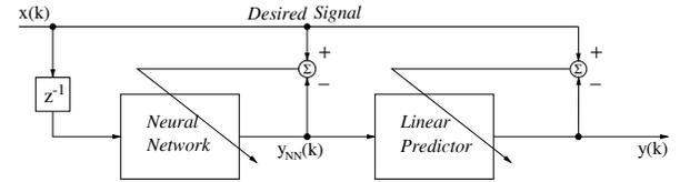
**Fig. 1.** A hybrid filter for prediction: A temporal neural network followed by an FIR filter.
