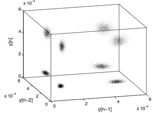
**Fig. 1.** 3D constellation of PMD channel. The data is from the simulation of a first order PMD channel with parameters given by: return-to-zero (RZ) Gaussian pulse, Peak power=2mW, Bit duration=100ps, Full width at half maximum (FWHM)=50ps, DGD=50ps,  $\gamma=0.5$  and the signal to noise ratio (SNR)=5.7dB.
