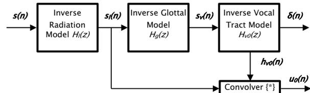
**Figure 6.** Estimation of the vocal tract inverse transfer function by coupled model inverter and convolver.
