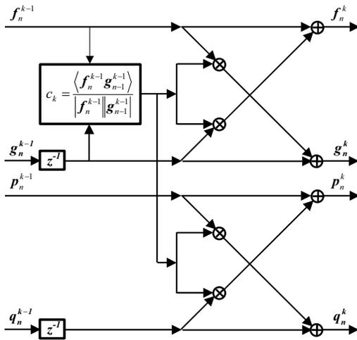
**Figure 8.** Coupled model inverter and convolver implemented by paired lattices.
