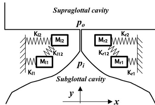
Figure 1. Schematic structure of the two-mass model.
