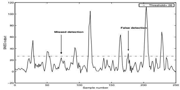
**Fig. 5.** The SNEO output to signal represented in Fig. 2(b)
