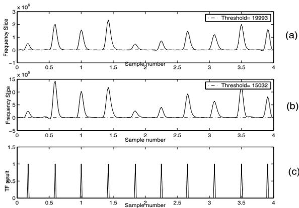
**Fig. 7.** Spike detection results using the TF-based technique applied on signal in Figure 6: (a) The first extracted frequency slice, (b) The Second extracted frequency slice, (c) The TF detector's output.
