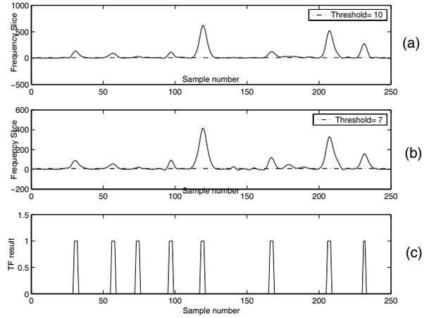
**Fig. 4.** TF spike detection on signal represented in Fig. 2b: (a) Frequency slice at  $l_F = \frac{5F_s}{12}$ , (b) Frequency slice at  $l_F = \frac{F_s}{2}$ , (c) Detection results.
