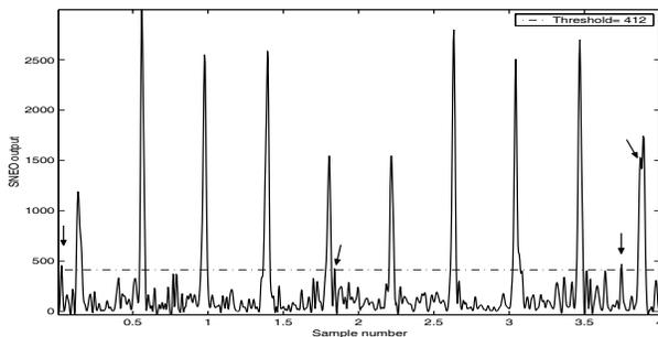
**Fig. 8.** The SNEO detector's output for signal represented in Fig. 6. False detected spikes are depicted by arrows.
