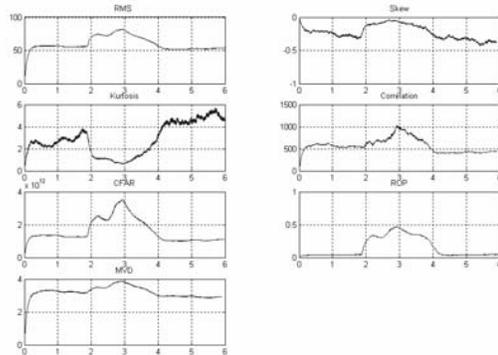
Figure 3 – Results for Test 5 – ABNT 1045 steel with severe burn from close to the beginning to the end of the workpiece; Horizontal axis corresponds time in seconds and Vertical axis Volts multiplied by a constant
