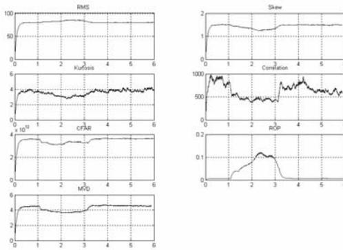
Figure 4 - Results for Test 7 – ABNT 1045 steel with burn in the midst of the part; Horizontal axis corresponds time in seconds and Vertical axis Volts multiplied by a constant
