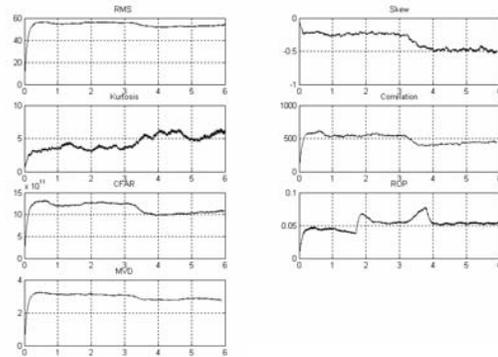
Figure 2 – Results for Test 1 – ABNT 1045 steel with no burn occurrence; Horizontal axis corresponds time in seconds and Vertical axis Volts multiplied by a constant
