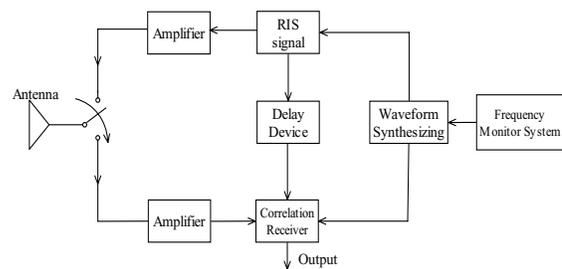
Fig.1. Block diagram of the RIS signal radar system
