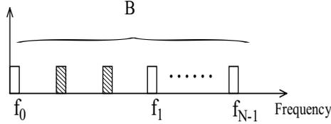
Fig.2 The frequency distribution of RIS signal waveform
