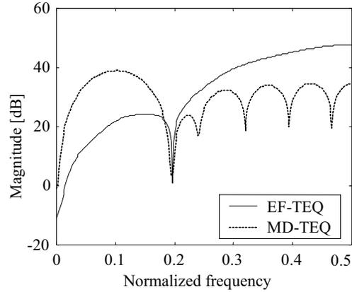
Fig. 10. Frequency response of two 16-tap TEQs designed for DMT system with narrowband interference of level  $-30$ dBm located in  $0.2f_s$ .
