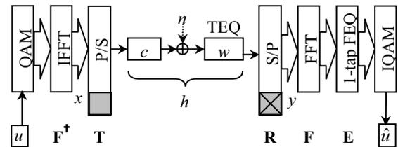
Fig. 1. Simplified block structure of DMT modem.
