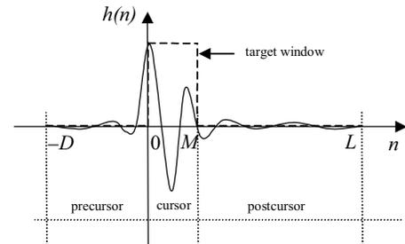
Fig. 2. Partition of shortened (time equalized) line impulse response  $\mathbf{h}$  from figure 1 having length  $K=D+L+1$ .  $M$  is the length of cyclic prefix. Negative indexing of precursor (delay) term is used for convenience.
