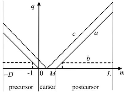
**Fig. 6.** Weighting sequences (see figure 2): a) ramp (proposed by the authors), b) wall (proposed in [4]), c) linear absolute (best solution in [4]).
