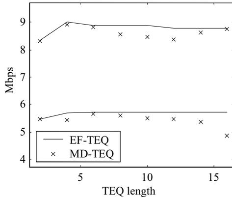
Fig. 8. Bit rate performance for different filter length in presence of AWGN of level  $-140$  dBm/Hz (upper two graphs) and  $-120$  dBm/Hz (lower two graphs).
