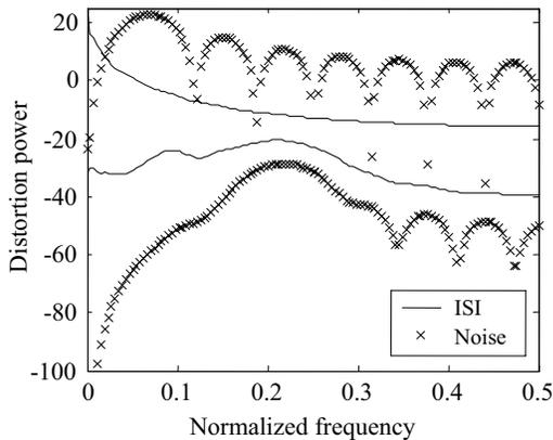
Fig. 9. Distortion power of ISI ( $P_{if}$ ) and Noise ( $P_n$ ) for MD-TEQ in presence of AWGN  $-100$  dBm/Hz (upper two graphs) and  $-160$  dBm/Hz (lower two graphs).
