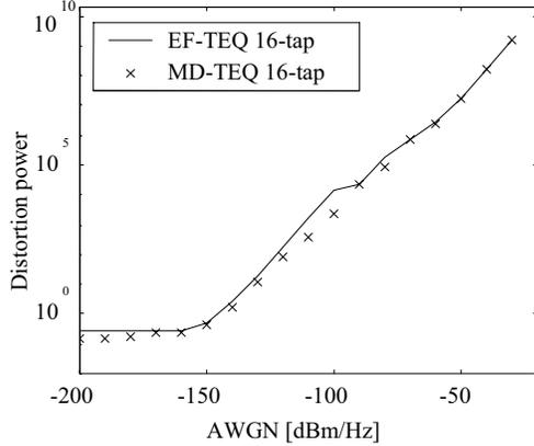
Fig. 7. Distortion power  $P_n + P_{if}$  for 16-tap equalizers.
