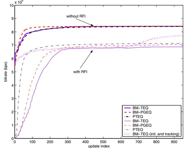
**Fig. 1.** Bitrate convergence of the BM-TEQ, BM-PGEQ (4 tone groups) and PTEQ, without (thin lines) and with RFI (thick lines).  $T = 32$ . The thick dotted line shows the adaptive BM-TEQ, initialized with an MMSE TEQ, tracking the disappearance of 2 RFIs at time instant 500.
