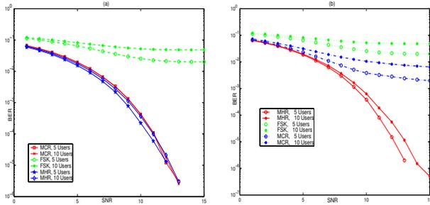
**Fig. 3.** Coherent MHR, MCR and FSK FH-CDMA in an AWGN channel with  $T_B = 4$  for 5 and 10 users. FM rates are chosen (a) to minimize MAI and (b) arbitrarily.
