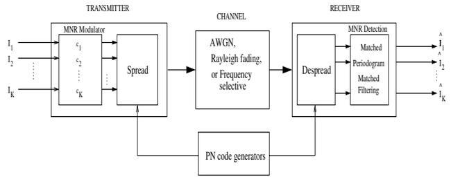
**Fig. 2.** MNR FH-CDMA system block diagram.
