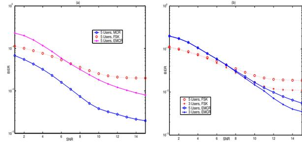
**Fig. 5.** Coherent MCR and FSK and estimated MCR (EMCR) FH-CDMA for an AWGN channel with (a)  $T_B = 4$ , and (b)  $T_B = 8$  and varying users.
