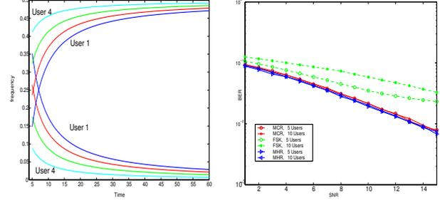
**Fig. 1.** (a) Unique HFMs of different users in the TF plane. (b) Performance comparison of coherent MHR, MCR and FSK FH-CDMA over a Rayleigh fading channel,  $T_B = 4$ .
