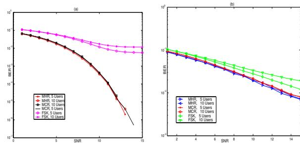
**Fig. 4.** Coherent MHR, MCR and FSK FH-CDMA with  $T_B = 1$  for 5 and 10 users. (a) AWGN channel, and (b) Rayleigh fading channel.
