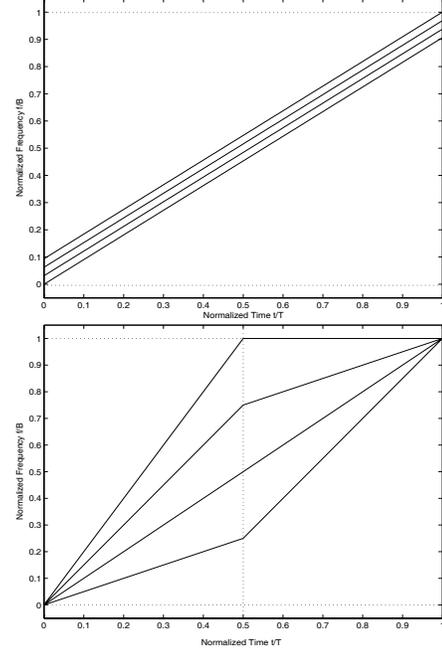
Fig. 2. Normalized IFs of modulating chirps of the proposed technique (top plot) and that proposed in [9]. Both systems are assumed to have the same time-bandwidth product  $TB = 32$  and the same number of users  $M = 4$ .
