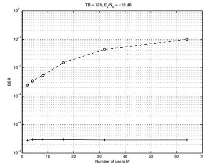
Fig. 4. BERs, as a function of  $M$ , of the proposed technique (continuous curve) and that in [9] (dashed curve) for  $TB = 128$  and  $SNR = -15$  dB.
