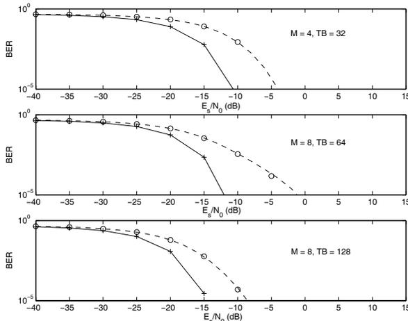
Fig. 3. BERs of the proposed technique (continuous curve) and that in [9] (dashed curve) for various values of  $TB$  and  $M$ .
