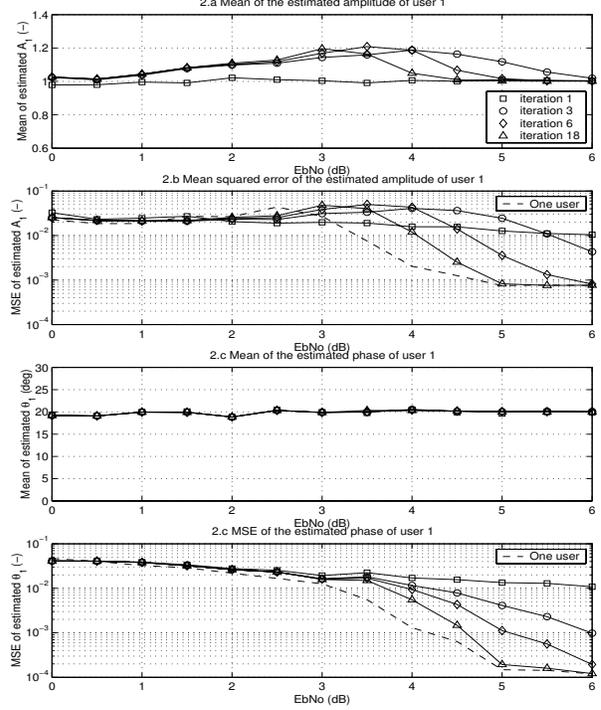
**Fig. 2.** Mean and mean-squared error of the amplitude and phase estimator versus  $E_b/N_0$ . User 1.
