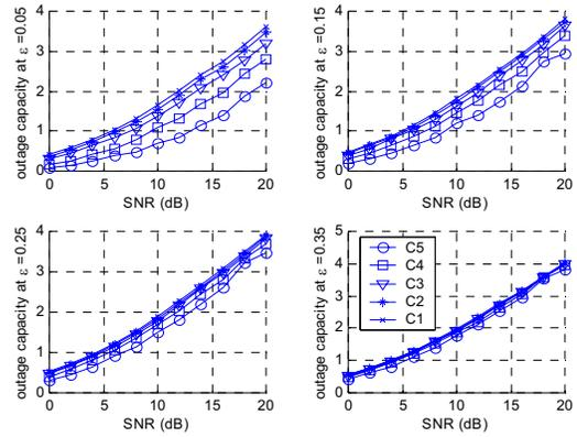
**Fig. 4.** Outage capacity vs. SNR. Traffic channel configurations are:  $C_1=\{(16, 1)\}$ ,  $C_2=\{(16, 2)\}$ ,  $C_3=\{(16, 4)\}$ ,  $C_4=\{(16, 8)\}$ ,  $C_5=\{(16, 16)\}$ .
