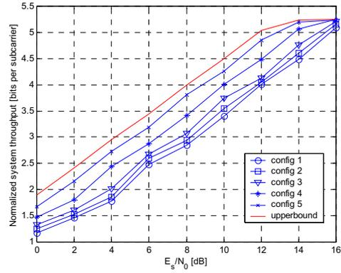
**Fig. 2.** Average normalized system capacity vs. SNR.  $K=64$ , TU channel and traffic channel configurations are:  $C_1=\{(16, 1)\}$ ,  $C_2=\{(16, 2)\}$ ,  $C_3=\{(16, 4)\}$ ,  $C_4=\{(16, 8)\}$ ,  $C_5=\{(16, 16)\}$ .
