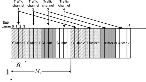
**Fig. 1.** Illustration of the traffic channel configuration:  $C=\{(8,4)\}$ .
