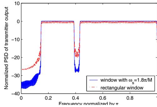
Figure 5: Comparison of the transmitter output power spectrum.
