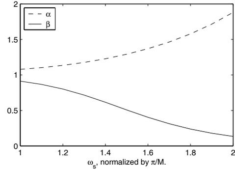
Figure 4: Plot of spectral leakage  $\beta$  and SNR loss  $\alpha$  as a function of stopband edge  $\omega_s$ .
