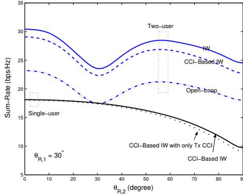
**Fig. 2.** Effects of the receiver-side spatial channel structure on the system sum-rate.
