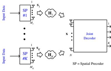
**Fig. 1.** Block diagrams of a MIMO MAC system.
