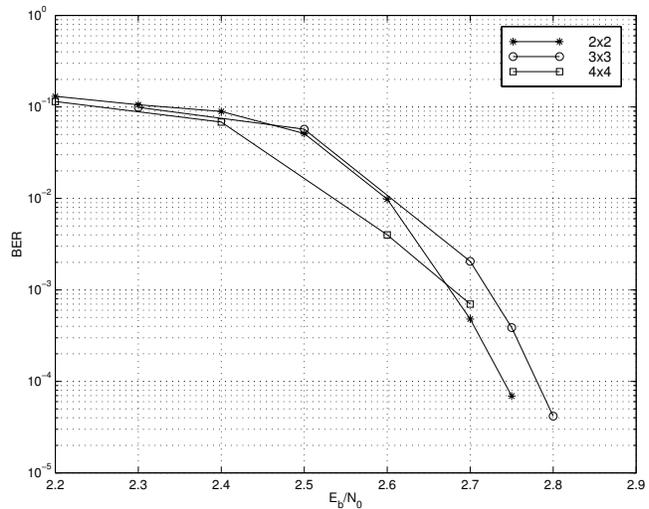
**Fig. 3.** Bit Error Rate of BICM using LDGM codes for QPSK and several (2x2,3x3 and 4x4) MIMO channels.
