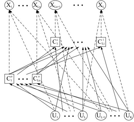
**Fig. 1.** Bayesian network representing the concatenated coding and modulation scheme.  $\{U_i\}$  represents the information bits,  $\{C_i^o\}$  the outer parity bits,  $\{C_i^i\}$  the inner parity bits and  $\{X_i\}$  the symbols transmitted through the channel.
