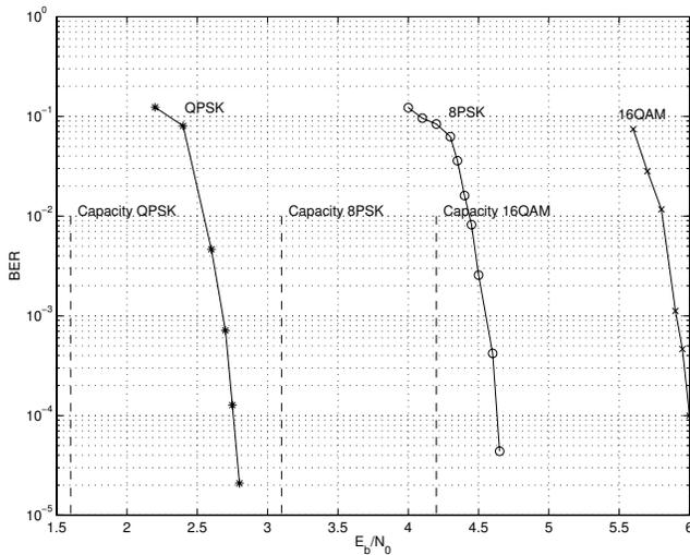
**Fig. 2.** Bit Error Rate of BICM using LDGM codes over a 2x2 MIMO channel
