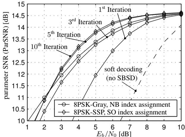
Fig. 5. Parameter SNR (ParSNR) for an AWGN channel
