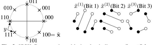
**Fig. 3.** 8PSK-Gray mapping with signal-pair distances  $\|y-\tilde{y}\|$  for  $\check{d}_h^{2(i)}(\mu)$ .  $\circ \leftrightarrow \tilde{x}^{(i)} = 0$  and  $\bullet \leftrightarrow \tilde{x}^{(i)} = 1$ .
