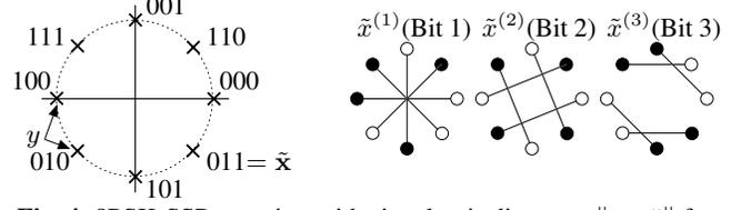
**Fig. 4.** 8PSK-SSP mapping with signal-pair distances  $\|y-\tilde{y}\|$  for  $\check{d}_h^{2(i)}(\mu)$ .  $\circ \leftrightarrow \tilde{x}^{(i)} = 0$  and  $\bullet \leftrightarrow \tilde{x}^{(i)} = 1$ .
