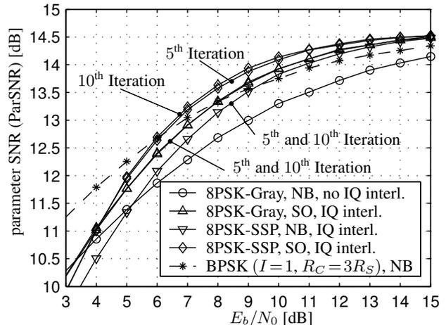
Fig. 6. Parameter SNR (ParSNR) for a Rayleigh channel
